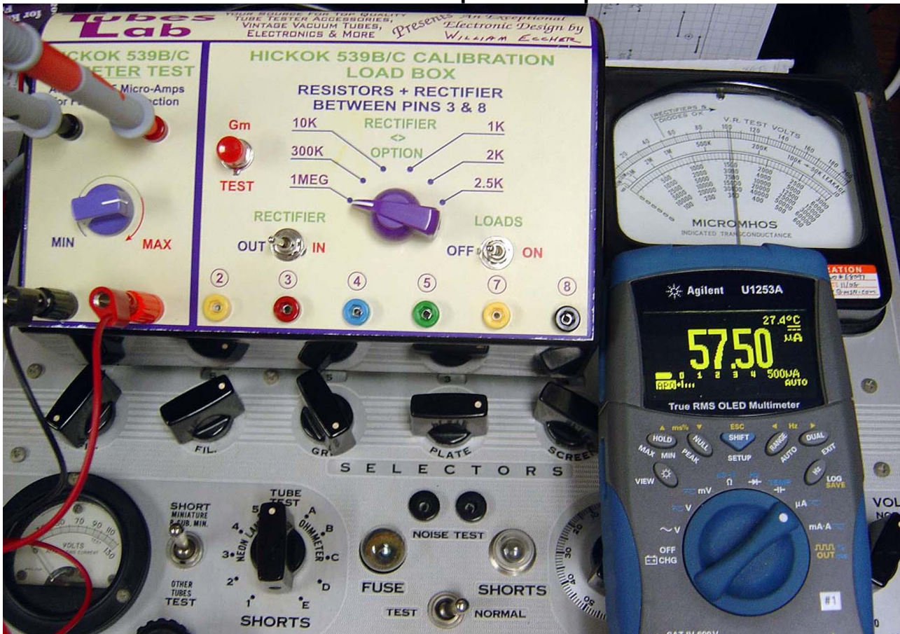
This picture shows the Main Meter reading 1/2 of full scale and with the Digital Multimeter indicating 57.5 microamps
